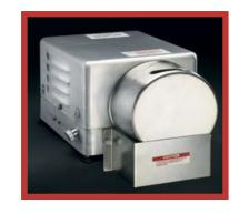
We manufacture the "**PRAWNTO** $^{\text{TM}}$  shrimp cutter and devein, the most dependable piece of equipment of its kind on the market today. Because it is powered by a ¼ hp motor and constructed of aluminum and stainless steel, and high quality standards are used in the manufacturing processes, we offer a 1-year warranty.
